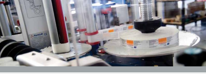
**Labellers** are specifically designed and customisable to customer requirements and are available in a number of configurations including single, or twin labelling heads with PLC control and interlocked glass/polycarbonate guarding as optional extras.
